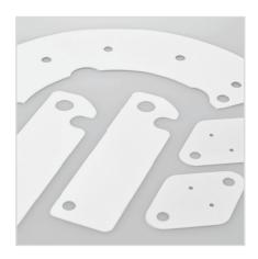
The highly thermaoconductive white group, with its well-balanced thermal, electrical and dielectric behaviour and very good self-adhesion characteristics, is created by filling a silicone elastomer base with aluminum oxide. An increase in mechanical strength can be achieved through fibre glass reinforcement. These film types can optionally be supplied with an additional adhesive coating.
