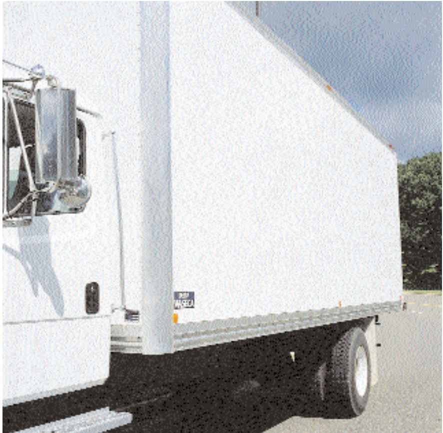
Smooth trucking – 3M™ VHB™ Tape replaced rivets in bonding truck side panels to stiffeners. The result was a much smoother, cleaner appearance and a strong bond. In addition to the design improvement, VHB tape can reduce vibration in the box.
