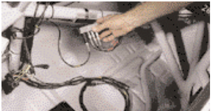
Fast Attachment – 3M™ Dual Lock™ Reclosable Fastener secures a telemetry transponder in this NASCAR stock car. The transponder is easily removed on race day.
