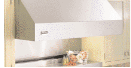
Replacing spot welds – In this range hood application, 3M™ Structural Bonding Tape replaced spot welding. The tape provides the strength of welding while sealing edges and preventing leaks. The use of tape also eliminated refinishing the steel after welding.
