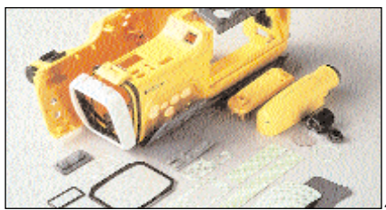
Die-cut for easy assembly – For assembly efficiency, die-cut pieces of 3M™ VHB™ Tape bond components in a water-resistant video camera case. The foam conforms to help seal the unit.
