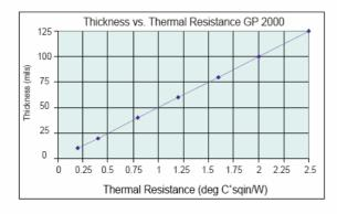
The resultant thickness of the Gap Pad will determine the thermal resistance. Subtracting the initial gap pad thickness by the deflection value, obtained above, will give the resultant thickness. Refer to the second graph to obtain the thermal resistance for a given thickness of material.
