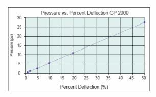
To calculate the approximate amount of deflection for a specific material thickness, at a given pressure, refer to the graph above. Multiply the thickness of the material by the percentage at the given pressure.\*
