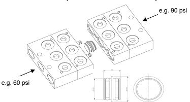
By adding this special plug, two different air pressures can be supplied to the same modular manifold plate.
