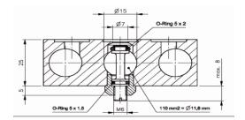
Certain applications require to plug the air supply one any valve of the plate individually. To meet that requirement, we developed the "D1-elements" for our 5 way assemblies.
