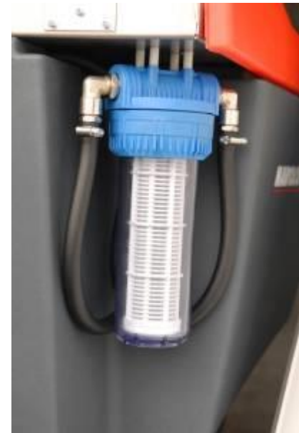
Washable and reusable 50µ easy access cartridge filter.
